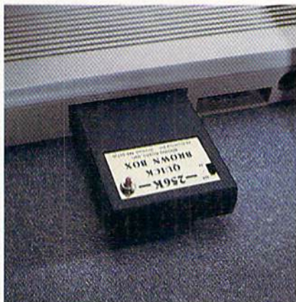
QBB is the grandfather of RAM expansion. Non-volatile memory sets it apart.
