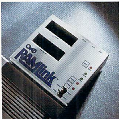
RAMLink is the "everything" box: extra RAM, an interface and an expansion port.
