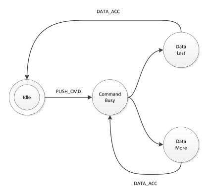
**Figure 1: Basic Protocol State Machine**
